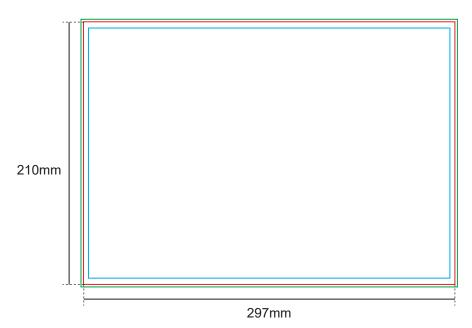
\* Safe zone = 5mm is applicable for panel size for perforation, creasing and folding. For panel size less than safe zone area, for example minimum creasing panel = 4mm, it is not advice to put important item into the panel.
