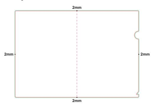
▶ Safe Zone : **5mm** for top, left & right edges. While **10mm** for bottom edge.
